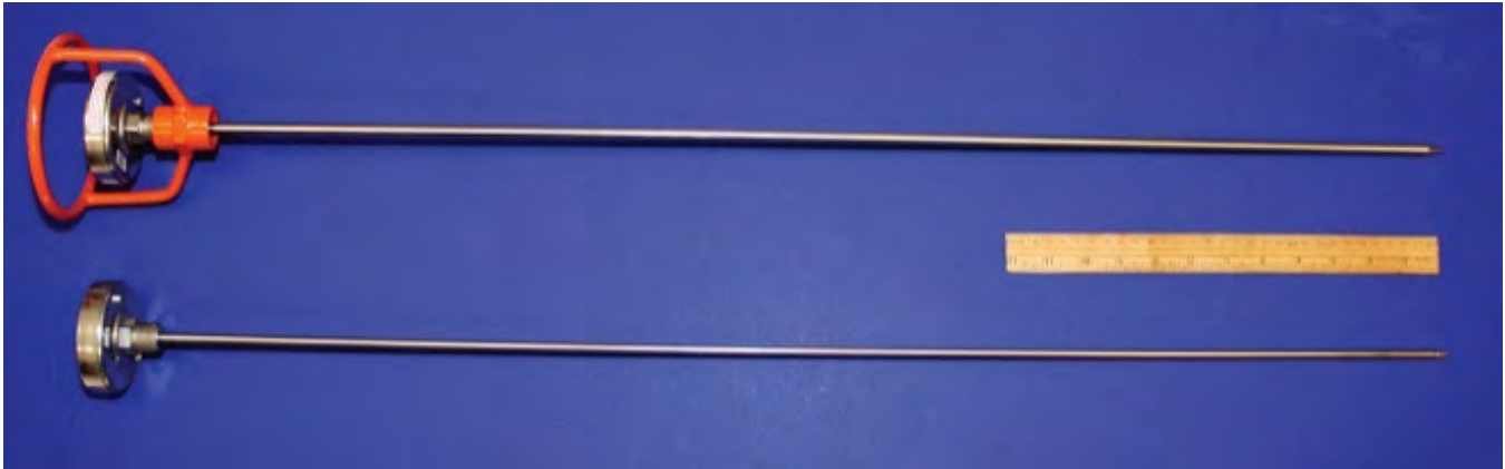
Photograph 1. Compost thermometers are 3 to 4 feet long.
